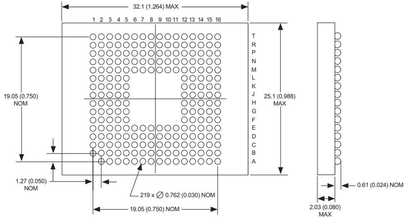
ALL LINEAR DIMENSIONS ARE MILLIMETERS AND PARENTHETICALLY IN INCHES
