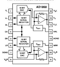
The AD1868 operates on +5 V power supplies. The digital supply, V<sub>L</sub>, can be separated from the analog supply, V<sub>S</sub>, for reduced digital feedthrough. Separate analog and digital ground pins are also provided. In systems employing a single +5 volt power supply, V<sub>L</sub> and V<sub>S</sub> should be connected together. In battery operated systems, operation will continue even with reduced supply voltage. Typically, the AD1868 dissipates 50 mW.
