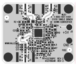
CV110-2A: The application circuit can be broken up into four main functions as denoted in the colored dotted areas above: RF/IF diplexing (purple), amplifier matching (green), filtering (red), and dc biasing (blue). There are various placeholders for chip components in the circuit schematic so that a common PCB can be used for all WJ single-branch converters. Additional placeholders for other optional functions such as filtering are also included.
