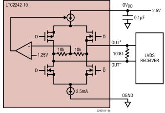
Figure 13b. Digital Output in LVDS Mode
