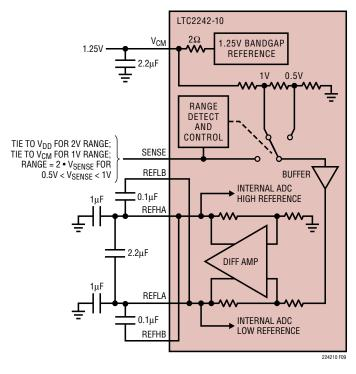
Figure 9. Equivalent Reference Circuit
