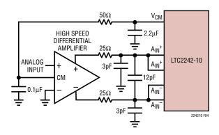
Figure 4. Differential Drive with an Amplifier
