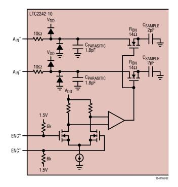
Figure 2. Equivalent Input Circuit
