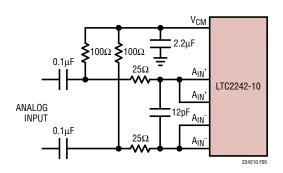
Figure 5. Capacitively-Coupled Drive
