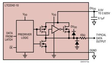
Figure 13a. Digital Output Buffer in CMOS Mode
