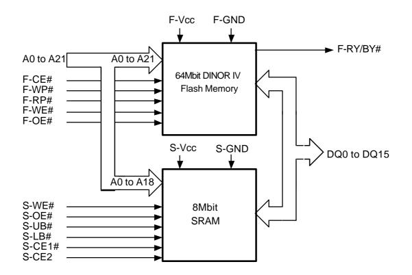
Note: In the Flash memory part there are "Vcc", "GND", "OE#" and "WE#" which mean "F-Vcc", "F-GND", "F-OE#" and "F-WE#", respectively. In the SRAM part there are "GND", "UB#", "LB#", "OE#" and "WE#" which mean "S-GND", "S-UB#", "S-LB#", "S-OE#" and "S-WE#", respectively.
