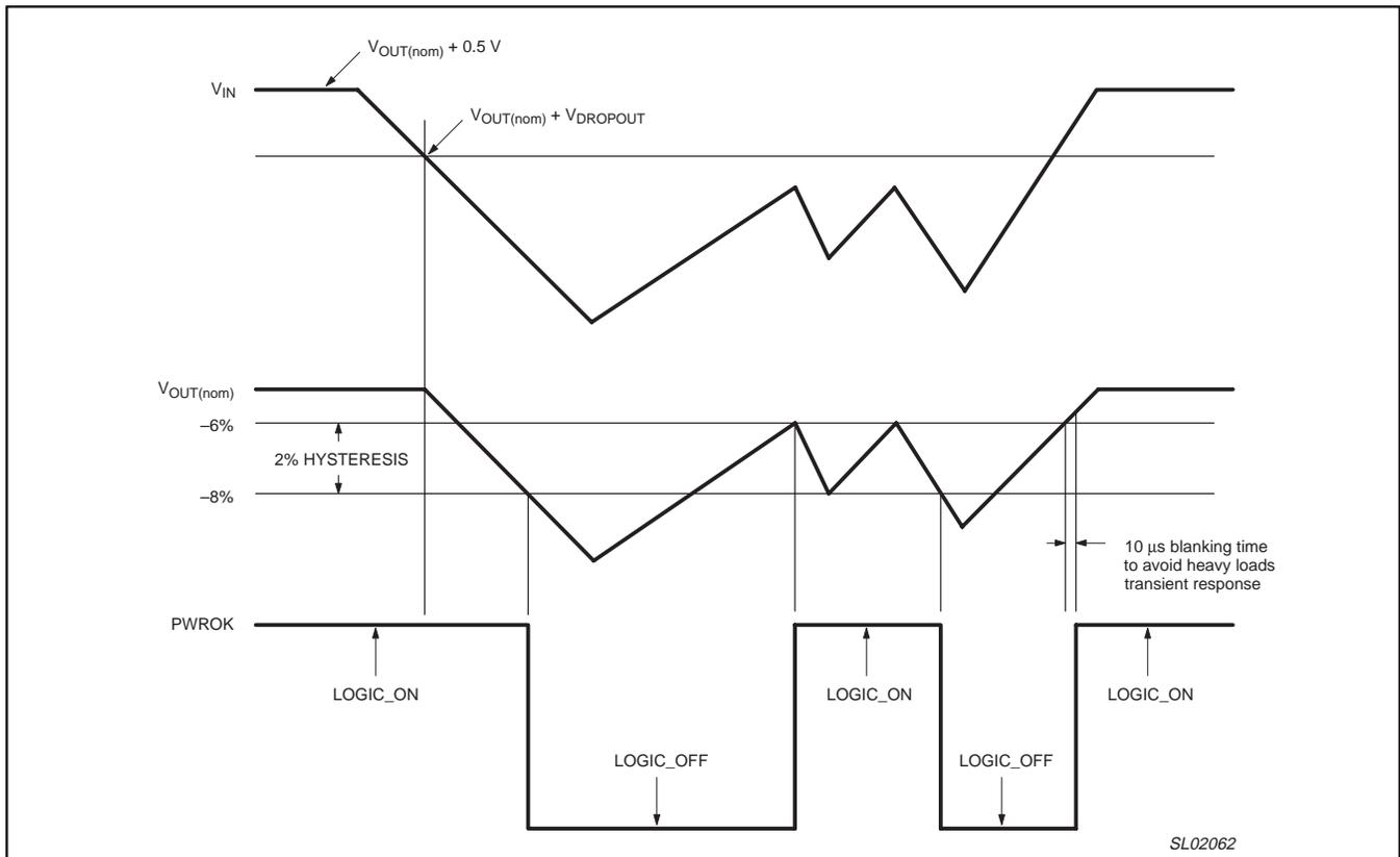
Figure 8. Timing diagram.
