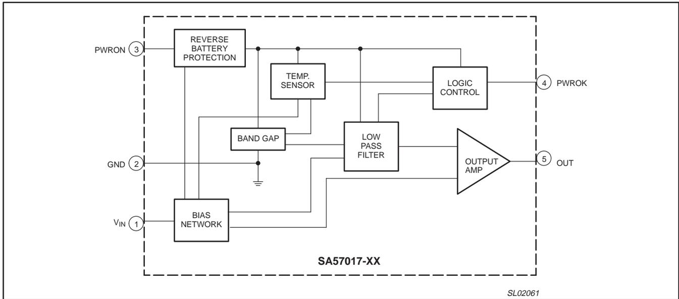
Figure 7. Simplified block diagram.
