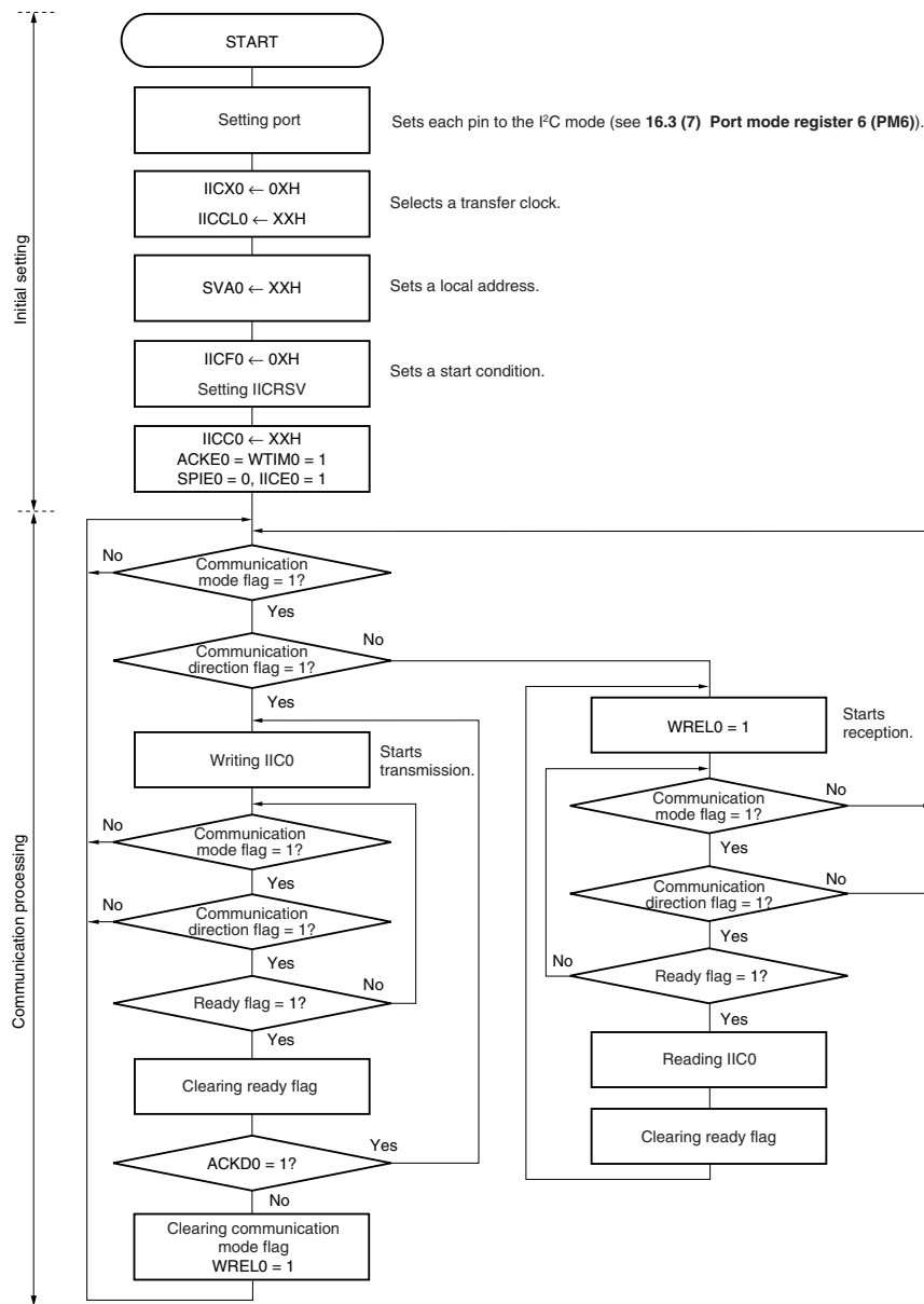
Figure 16-25. Slave Operation Flowchart (1)
