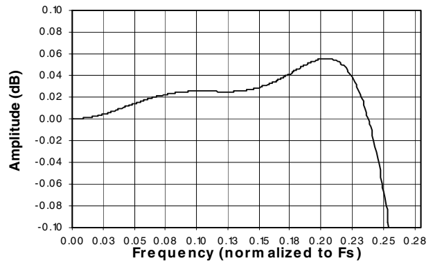
Figure 12. Quad Speed Passband Ripple
