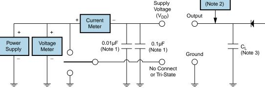
Note 1: An external 0.1µF low frequency tantalum bypass capacitor in parallel with a 0.01µF high frequency ceramic bypass capacitor close to the package ground and V<sub>DD</sub> pin is required.
