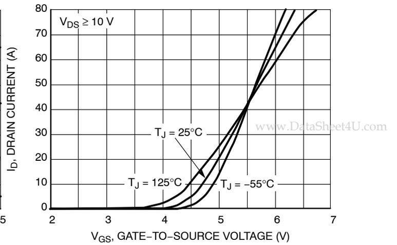
Figure 2. Transfer Characteristics
