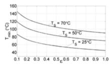
Graph showing the minimum measuarable object temperature  $(T_{min})$ , determined by surface emissivity  $(\epsilon)$  and sensor temperature  $(T_S)$ .
