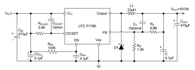
Note:  $V_{OUT} = V_{FB} x (1+R_A/R_B)$ ,  $R_B$ =0.7K~5K ohm
