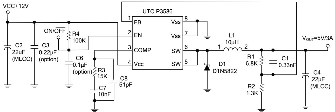
Notes:  $V_{OUT} = V_{FB} \times \left( \frac{R1 + R2}{R2} \right)$
