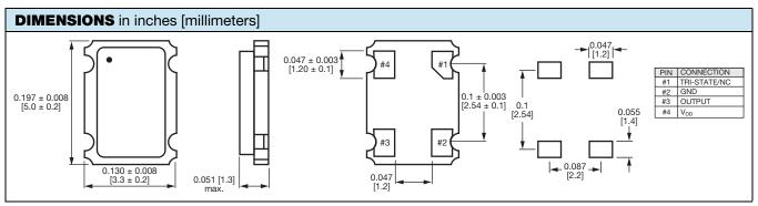
A 0.01 μF bypass capacitor should be placed between V<sub>DD</sub> (pin 4) and GND (pin 2) to minimize power supply line noise
