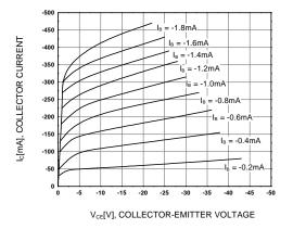
Figure 1. Static Characteristic
