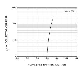
Figure 4. Base-Emitter On Voltage
