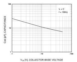
Figure 5. Collector Output Capacitance
