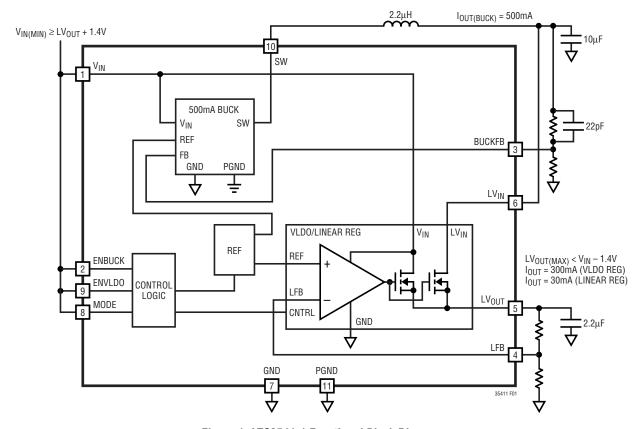
Figure 1. LTC3541-1 Functional Block Diagram
