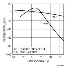
Figure 9. Change in Capacitor vs Temperature
