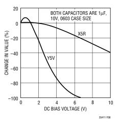
Figure 8. Change in Capacitor vs Bias Voltage
