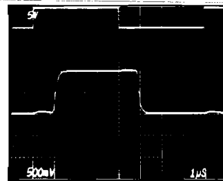
MUX-24 SMALL-SIGNAL SWITCHING WITH FILTERING
