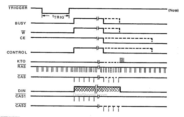
Note: The TRIGGER pin is normally connected to the telephone ringer detector t<sub>TRIG</sub> means the time duration after the first signal is on. If pause time between two ringer signals exceeds 4 seconds, the trigger duration will reset to zero. The trigger shown below works, where t<sub>TRIG</sub> ≥ 10.75 seconds and pause time (t1, t2, t3) must be less than 4 seconds.
