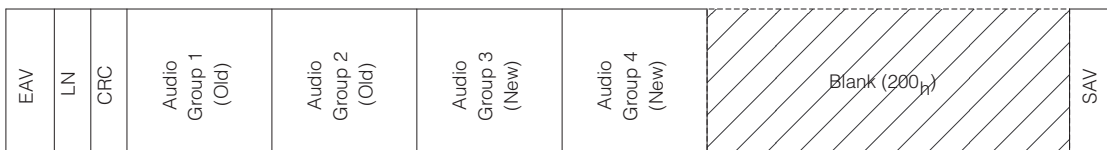
Video Signal after GS1503B Insertion of Audio Groups 3 & 4 (CASCADE = 1)
