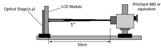
[Figure 8] Optical characteristic measurement equipment and method
