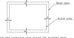
7. Do not wind conductive tape around the backlight wires 8. Gap between Bezel and Panel : Max 0.7mm
