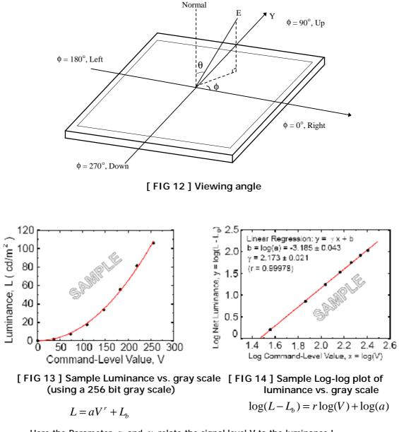
Here the Parameter  $\alpha$  and  $\gamma$  relate the signal level V to the luminance L. The GAMMA we calculate from the log-log representation (FIG. 7)
