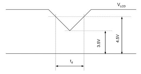
[Figure 7] Power dip condition
