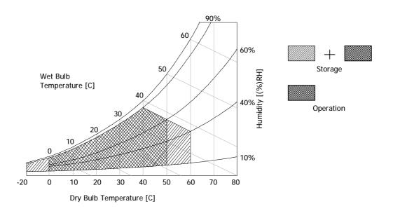
[Figure 2] Temperature and relative humidity
