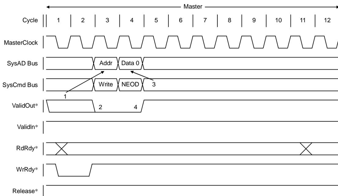
Figure 11.2.13 Processor Non-coherent Single Word Write Request Protocol
