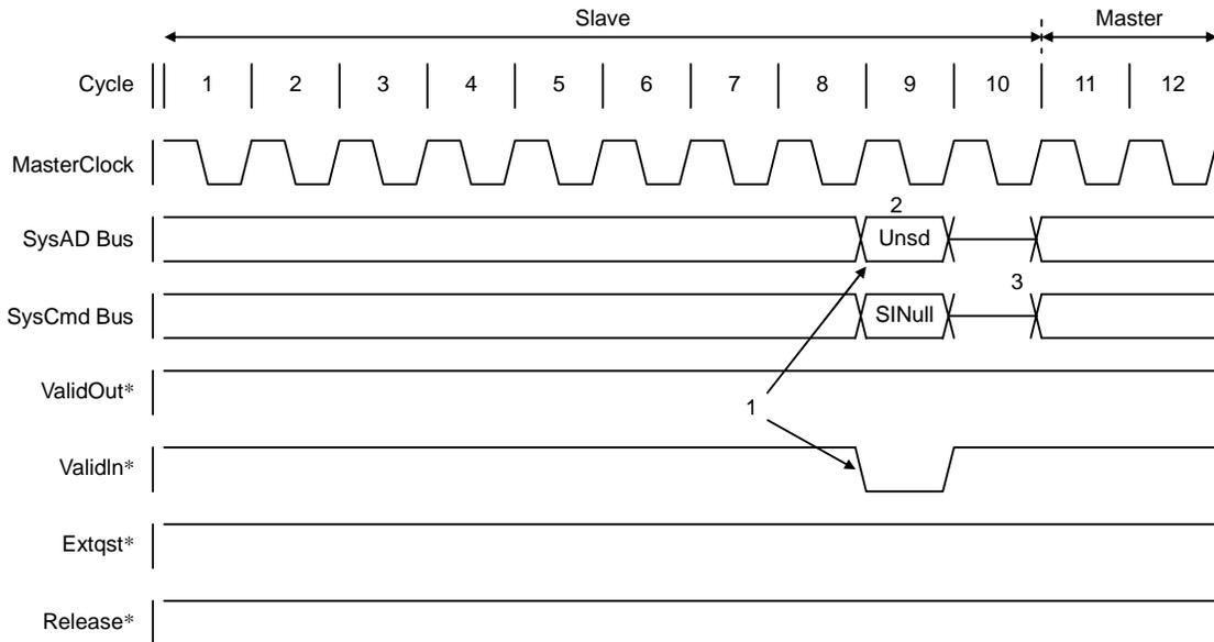
Figure 11.2.20 System Interface Release External Null Request
