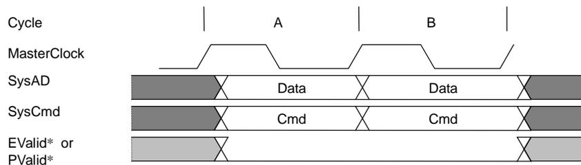
Figure 11.3.7 Sample Cycles with Multiple PValid\* and EValid\*
