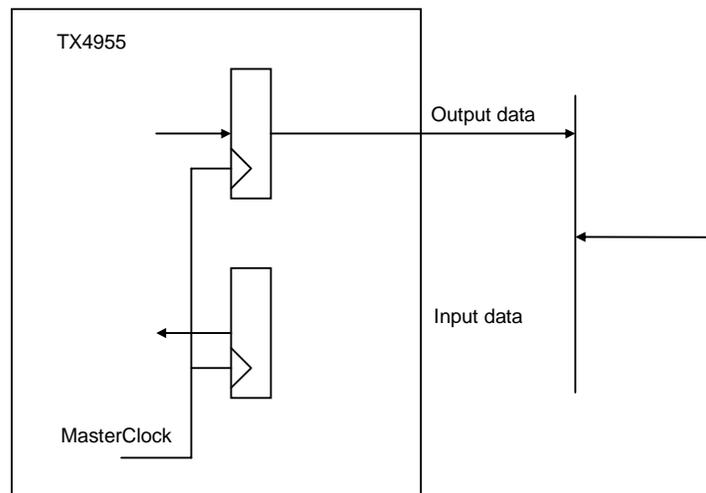
Figure 11.2.4 Operation of the System Interface Between Registers
