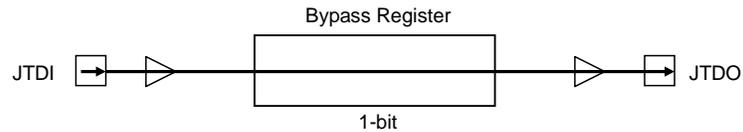
Figure 14.4.4 Test Data Flow While the Bypass Instruction is Selected
