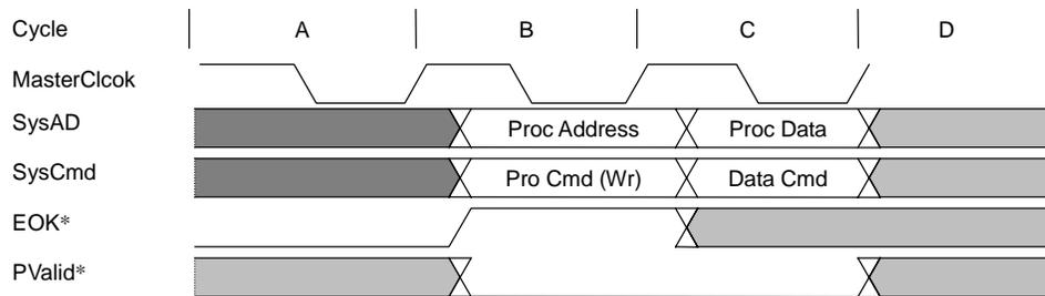
Figure 11.3.9 Sample Cycle with EOK\* Asserted, Then Deasserted
