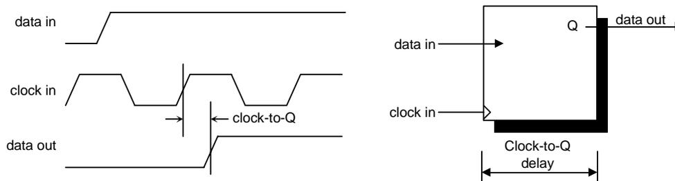
Figure 10.1.2 Clock-to-Q Delay
