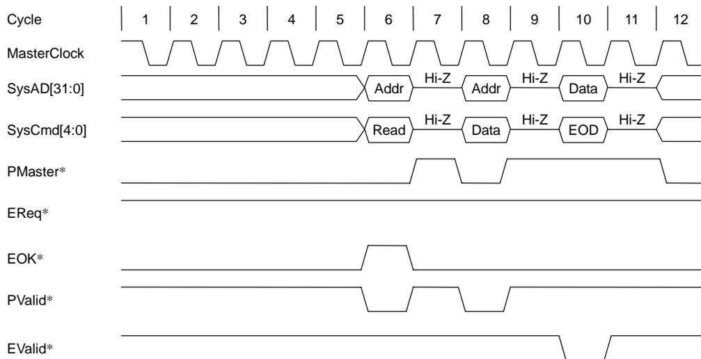
Figure 11.3.30 Discarding and Re-executing Processor Single Read Request
