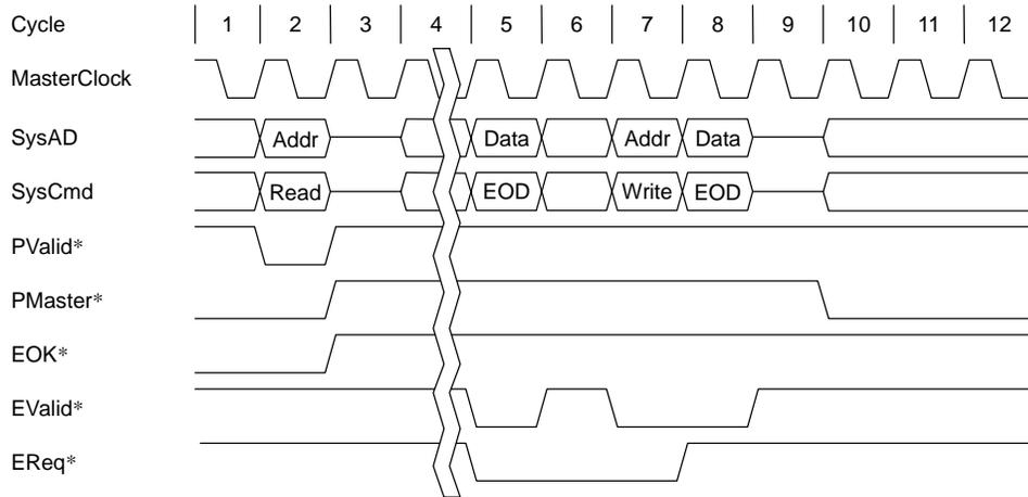
Figure 11.3.20 Single Read Request Followed By External Write Request
