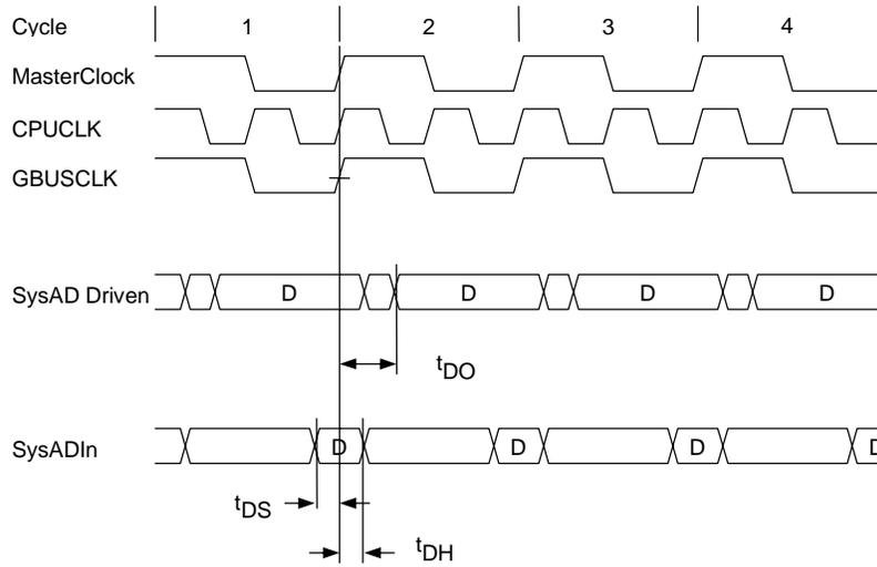
Figure 10.2.2 Processor Clock, CPUCLK-to-GBUSCLK Divisor of 2
