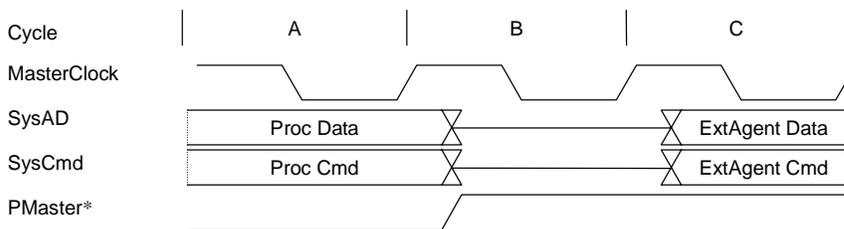
Figure 11.3.4 Sample Cycle with PMaster\* Asserted, Then Deasserted
