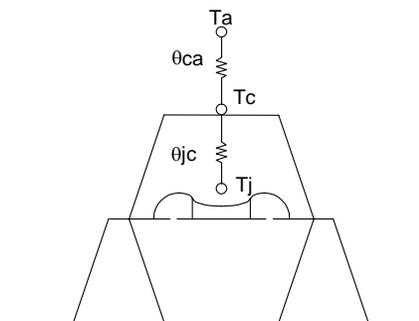
**Figure 3.2 Thermal Resistance of Package**
