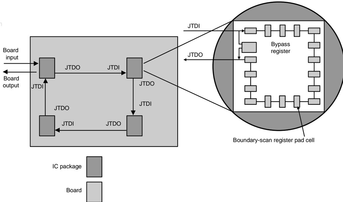
Figure 14.3.3 Bypass Register Operation
