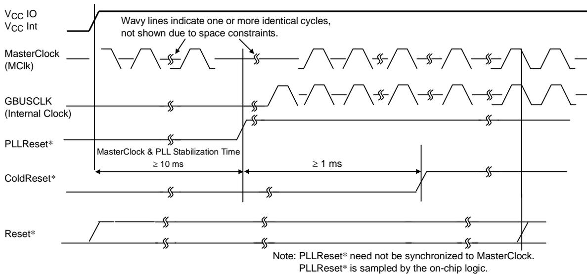
Figure 9.2.1 Power-On Reset Timing
