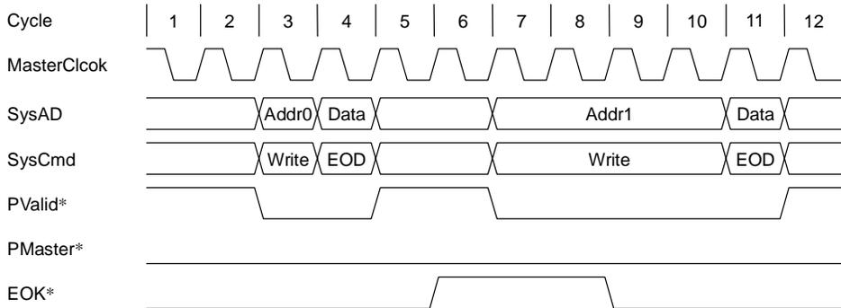
Figure 11.3.23 Two Processor Write Requests, Second Write Delayed
