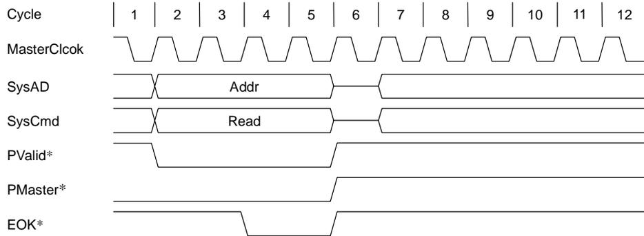
Figure 11.3.22 Delayed Processor Read Request
