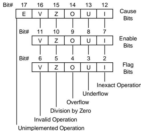
Figure 3.3.4 Control/Status Register Cause, Flag, and Enable Fields
