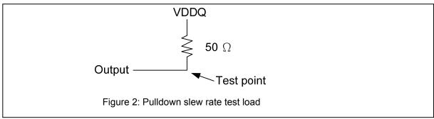
c. Pullup slew rate is measured between (VDDQ/2 - 320 mV  $\pm$  250 mV)
