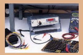
Even the best test instrument won't help you if you can't make the proper connections. Having a test lead that can access an IC pin without shorting, or a patch cord that accommodates multiple stacking, can make all the difference during a critical test.
