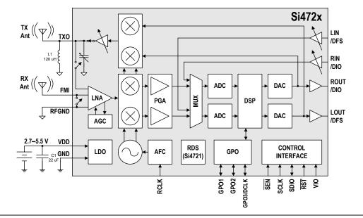
Si4720/21 Broadcast FM Radio Transceiver for Portable Applications
