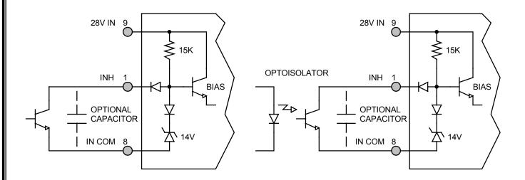
**Figure 4** – Internal Inhibit Circuit and Recommended Drive (Shown with optional capacitor for turn-on delay)
