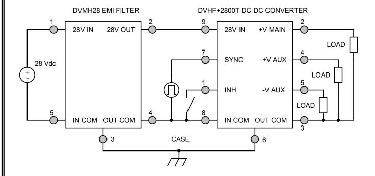
Figure 6 – Converter with EMI Filter
