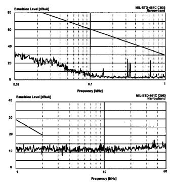
Figure 10 - DVHF+2800T with EMI Filter
