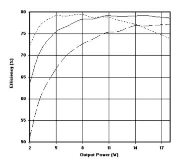
Figure 8 – DVHF+28515T Efficiency (%) vs. Output Power (W)
