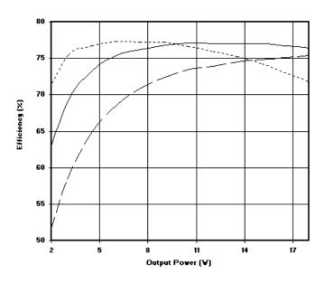
Figure 7 – DVHF+28512T Efficiency (%) vs. Output Power (W)
