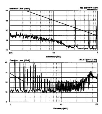
Figure 9 - DVHF+2800T without EMI Filter
