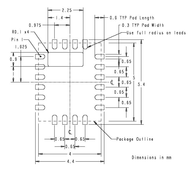
Figure 11. Recommended PCB Solder Mask Openings.
