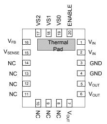
Figure 3. Pin description, bottom view.
