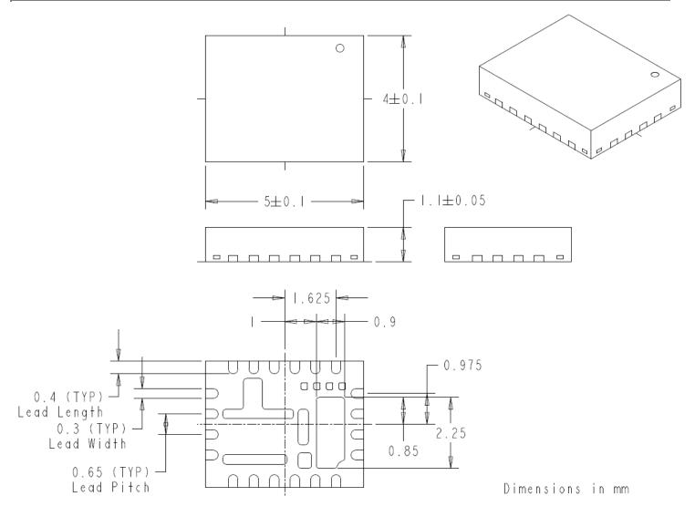
Figure 12. Package mechanical dimensions.
