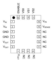
Figure 2. Pin description, top view.
