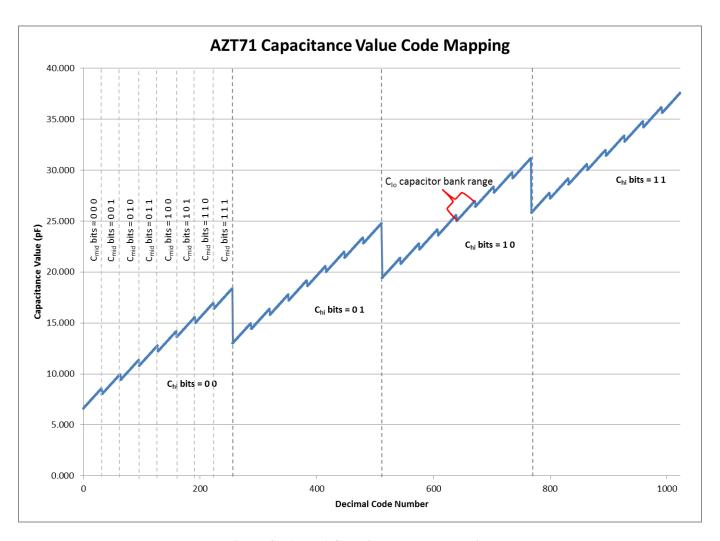
Figure 4 – AZT71 Capacitance Value Mapping
