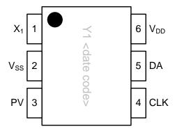
Figure 2 - Pin Configuration TSOT6
