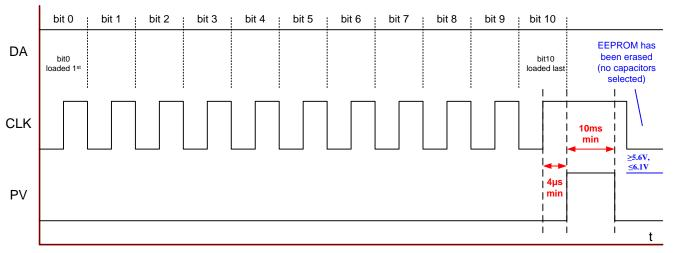
Figure 13 – Programming Sequence for erasing the EEPROM
