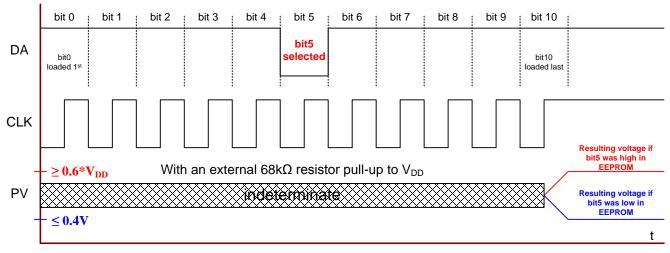
Figure 12 - Timing diagram to read bits from EEPROM
