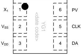
Figure 3 - Pin Configuration 6MLP
