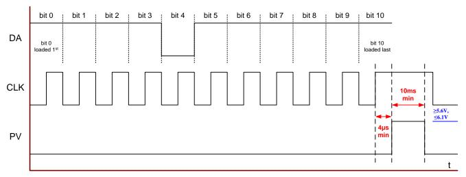
Figure 11 - Second programming cycle to program bit4 into the EEPROM
