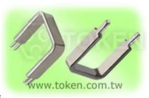
manufactured with 2 or 4 soldertags (terminals). The LPS type B with 2 soldertags (1 pin on each side) is a standard part of LPS series and type A with 4 terminals (2 pin on each side) is used either for Kelvin connections or for high current applications. Depending from the alloy material's thickness, one terminal contact on each side can carry up to 50A (A (Current) = (W (Power)/ $\Omega$  (Resistance))1/2), so a 4-terminal part can carry 100A (ask Token factory).
