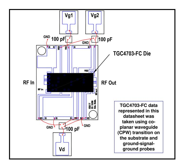
Die is flip-chip soldered to a 15 mil thick alumina test substrate
