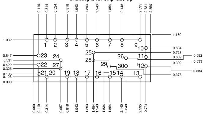
Units: millimeters Thickness: 0.380
