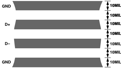
Figure 19. Arrangement of Signal Tracks
