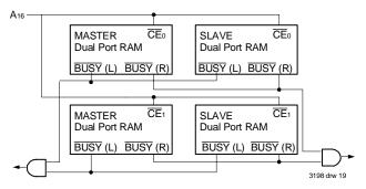
Figure 3. Busy and chip enable routing for both width and depth expansion with IDT7008 RAMs.
