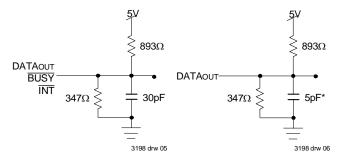
Figure 1. AC Output Test Load
