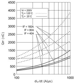
Fig. 8 - Typical Stored Charge vs. dl<sub>F</sub>/dt
