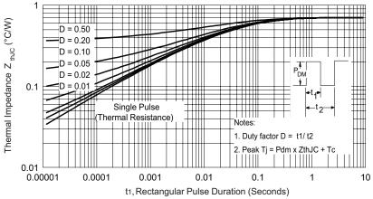
Fig. 4 - Maximum Thermal Impedance  $Z_{thJC}$  Characteristics
