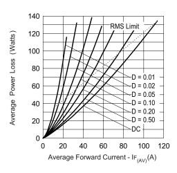
Fig. 6 - Forward Power Loss Characteristics
