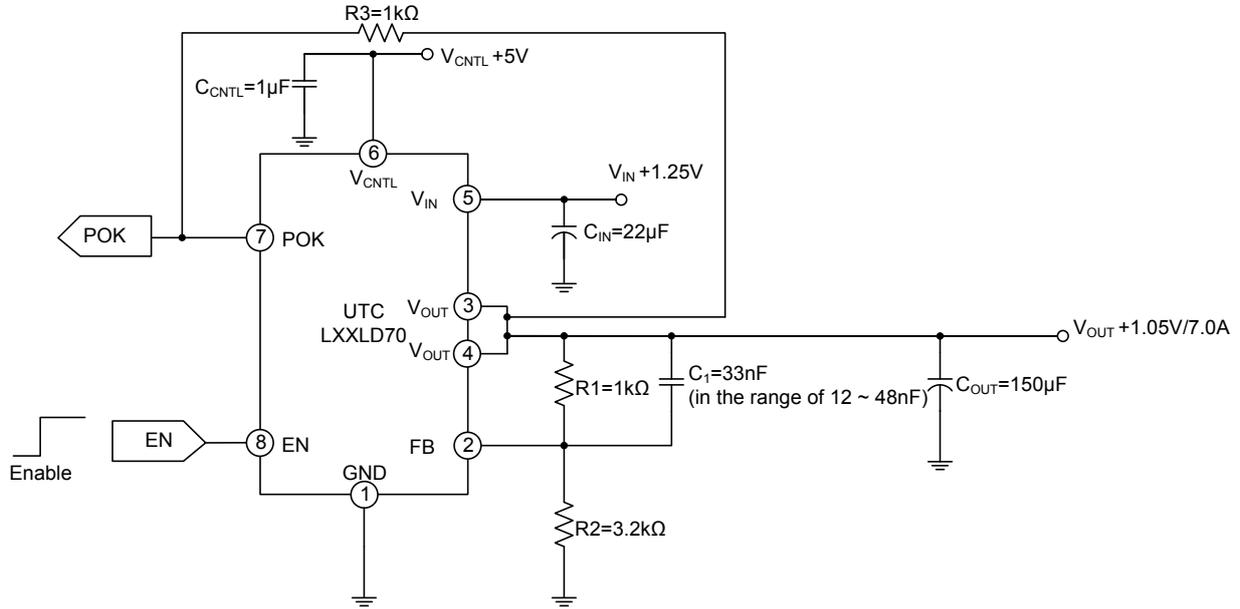
2. Using an MLCC as the Output Capacitor
