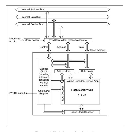
Figure 4.1.1 Block diagram of the flash unit
