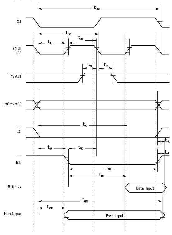
Note : The phase relation between X1 input signal and the other signals is unsettled. The timing chart above is an example.
