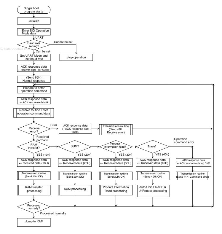
Figure 4.3.6 Overall flowchart for boot program
