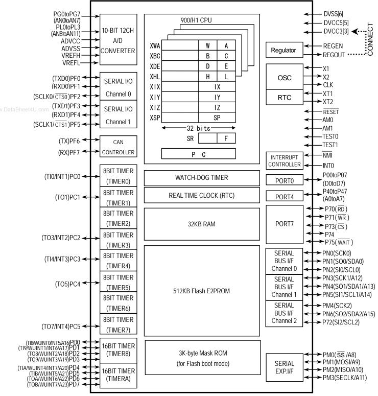
Figure 1 TMP92FD54AI block diagram
