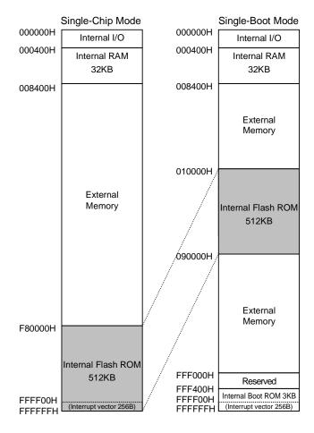
Figure 4.3.2 Memory maps for Single-Chip Mode and Single-Boot Mode
