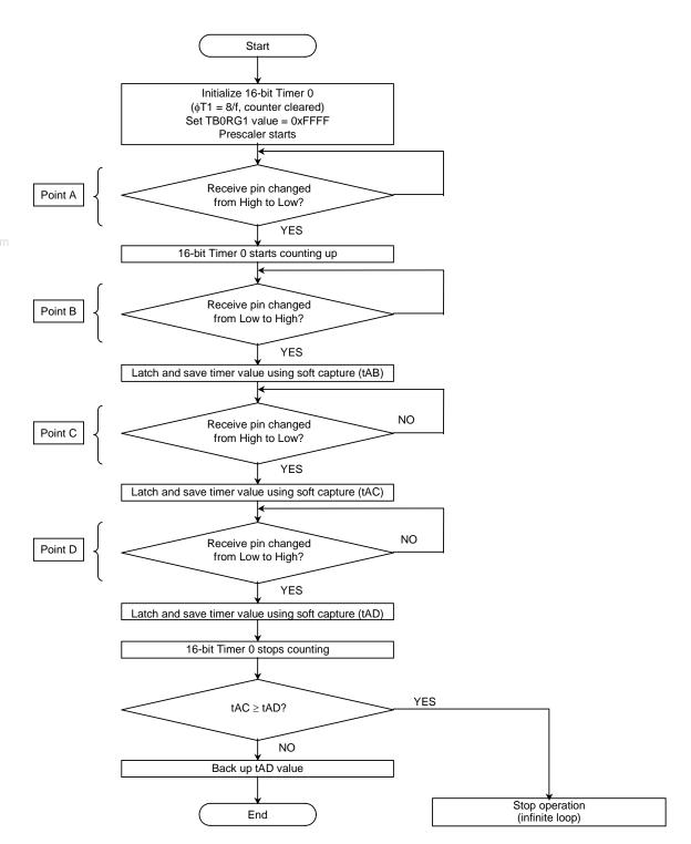
Figure 4.3.4 Serial operation mode reception flowchart
