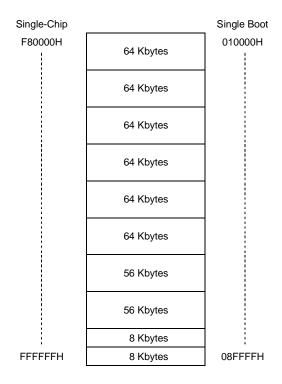
Figure 4.4.1 Flash memory block configuration
