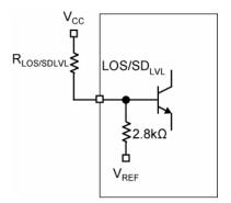
Figure 5. LOS/SDLVL Setting Circuit
