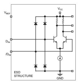
Figure 2. Input Structure
