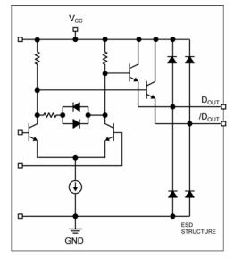
Figure 3. Output Structure
