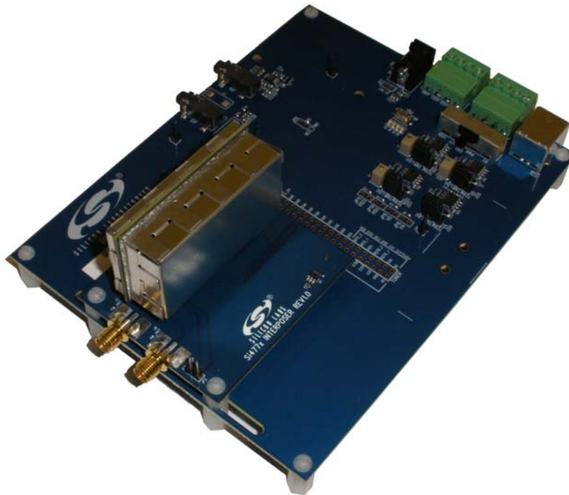
Figure 34. Si4770Module-A-EVB Module and Interposer Card
