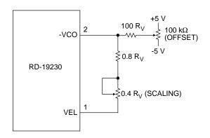
FIGURE 15. VELOCITY TRIMMING
