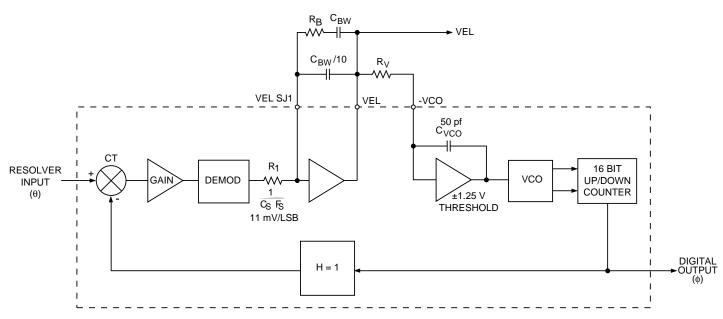
FIGURE 2. TRANSFER FUNCTION BLOCK DIAGRAM #1
