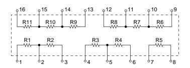
FIGURE 28. (DDC-49530, DDC-49590, DDC-57470) **LAYOUT AND RESISTOR VALUES (SEE TABLE 11)**
