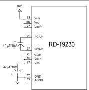
FIGURE 5. -5V INVERTER CONNECTIONS
