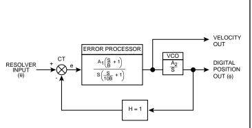
FIGURE 3. TRANSFER FUNCTION BLOCK DIAGRAM #2
