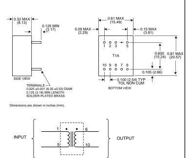
FIGURE 8. TRANSFORMER LAYOUT AND SCHEMATIC (REFERENCE INPUT - B-426)
