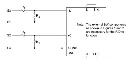
$$\frac{R_2}{R_1 + R_2} = \frac{2}{X \text{ Volt}}$$
