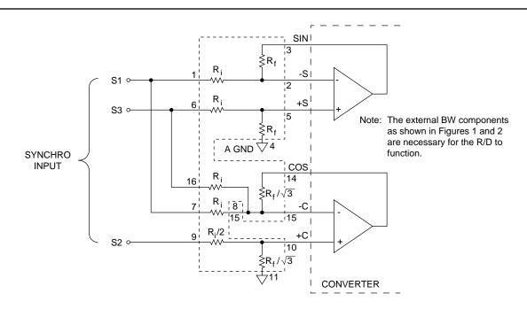
S1, S2, S3 should be triple twisted shielded; RH and RL should be twisted shielded;
