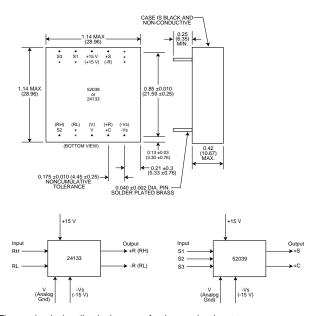
The mechanical outline is the same for the synchro input transformer (52039) and the reference input transformer (24133), except for the pins. Pins for the reference transformer are shown in parenthesis ( ) below. An asterisk \* indicates that the pin is omitted.
