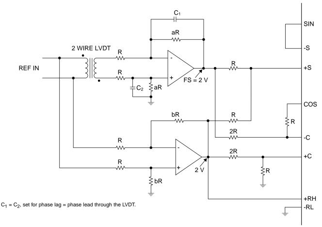
FIGURE 24, 2-WIRE LVDT DIRECT INPUT
