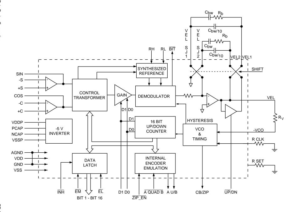
FIGURE 1. RD-19230 SERIES BLOCK DIAGRAM
