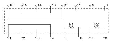
FIGURE 27. (DDC-55688) LAYOUT AND RESISTOR VALUES (R1 AND R2 = 10 K $\Omega$  1.0% TOL, ABSOLUTE TC = ±100 PPM MAX)
