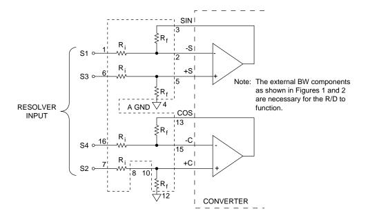
S1 and S3, S2 and S4, and RH and RL should be ideally twisted shielded, with the shield tied to GND at the converter. For DDC-49530:  $R_1 = 70.8 \text{ K}\Omega$ , 11.8 V input, synchro or resolver.
