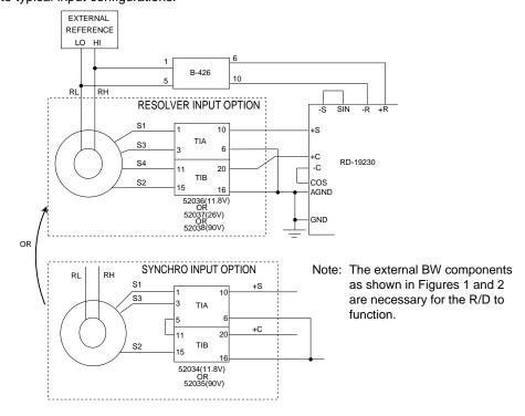
FIGURE 10. TYPICAL TRANSFORMER CONNECTIONS
