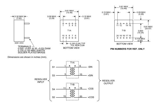
FIGURE 7. TRANSFORMER LAYOUT AND SCHEMATIC (RESOLVER INPUT - 52036/52037/52038)
