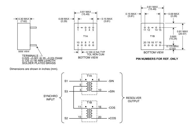
FIGURE 6. TRANSFORMER LAYOUT AND SCHEMATIC (SYNCHRO INPUT - 52034/52035)
