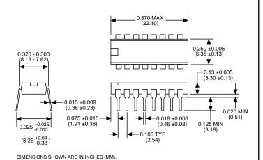
FIGURE 29. 16-PIN THIN-FILM RESISTOR NETWORK **DIP MECHANICAL OUTLINE** (DDC-49530, DDC-49590, DDC-55688)
