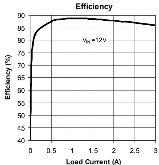
Figure 1. 350kHz 10V - 16V to 5V/3A Step-down Converter
