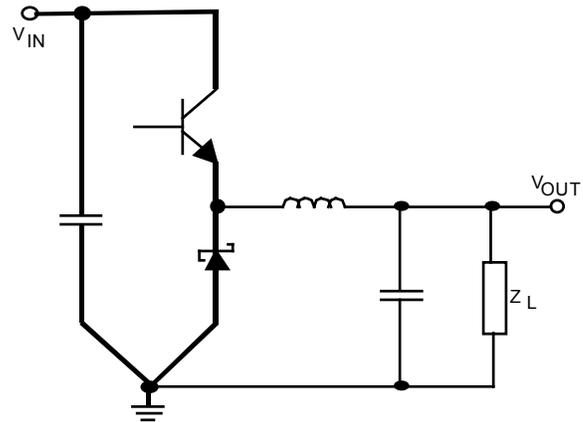
**Figure 9. Heavy lines indicate the critical pulse current loop. This stray inductance of this loop should be minimized.**
