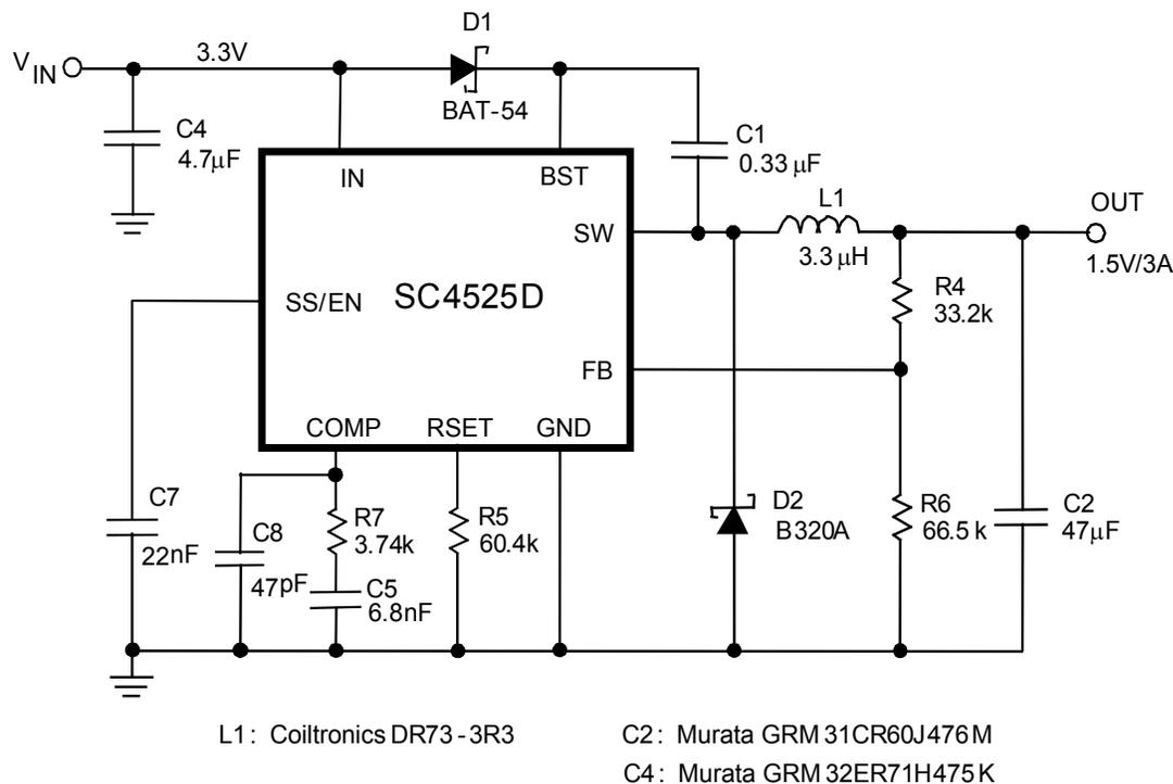
**Figure 11. 350kHz 3.3V to 1.5V/3A Step-down Converter**
