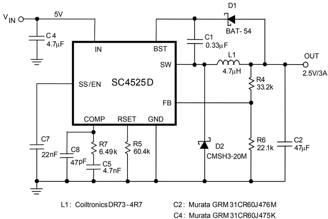
**Figure 10. 350kHz 5V to 2.5V/3A Step-down Converter**
