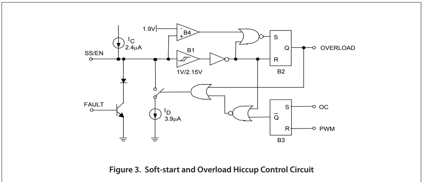
Figure 3. Soft-start and Overload Hiccup Control Circuit
