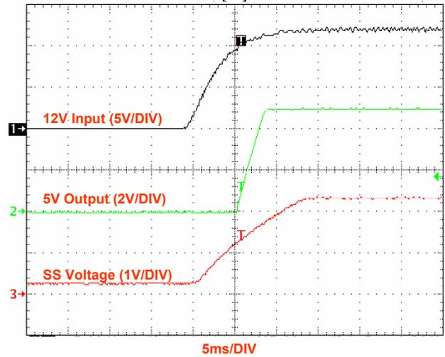
Figure 12(b).  $V_{IN}$  Start up Transient ( $I_O=3A$ )
