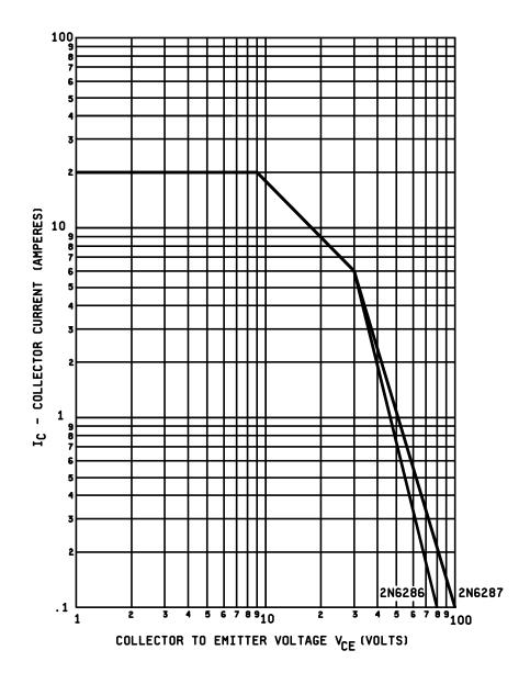
FIGURE 3. Maximum safe operating area (continuous dc).
