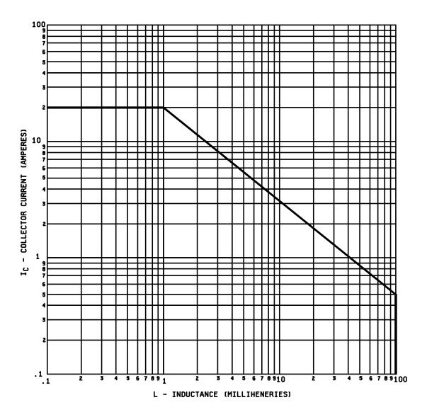
FIGURE 4. <u>Safe operating area for switching between saturation and cutoff</u> (unclamped inductive load).
