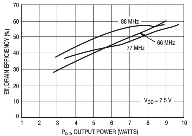
Figure 14. Drain Efficiency versus Output Power
