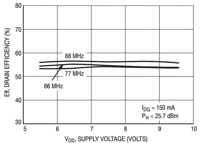
Figure 18. Drain Efficiency versus Supply Voltage
