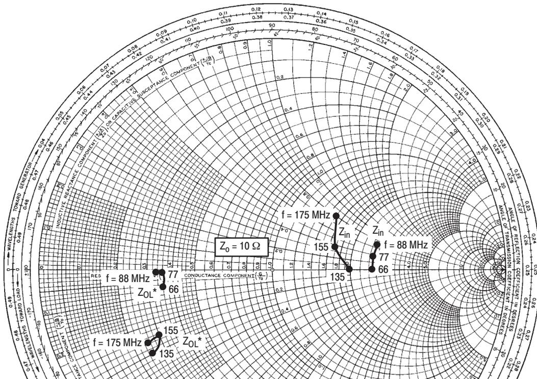
$V_{DD} = 7.5 \text{ V}$ ,  $I_{DQ} = 150 \text{ mA}$ ,  $P_{out} = 8 \text{ W}$
