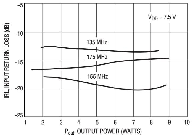
Figure 3. Input Return Loss versus Output Power
