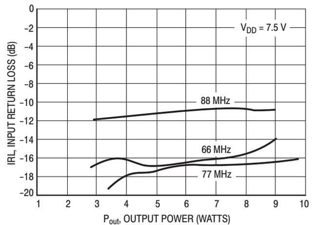
Figure 12. Input Return Loss versus Output Power
