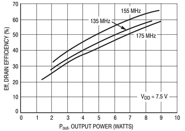
Figure 5. Drain Efficiency versus Output Power
