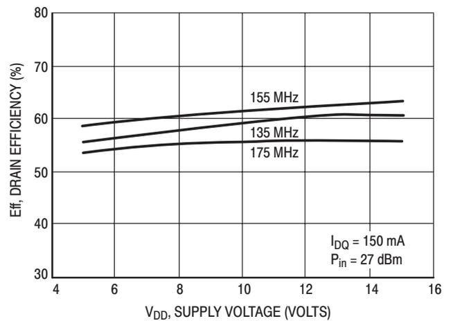
Figure 9. Drain Efficiency versus Supply Voltage
