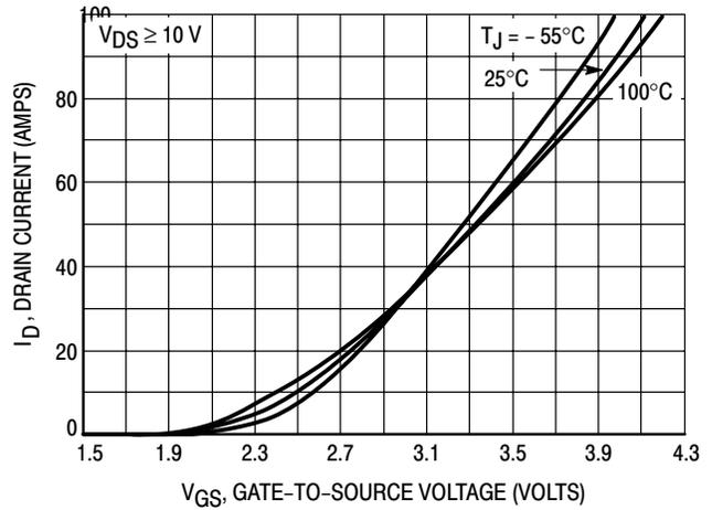
Figure 2. Transfer Characteristics
