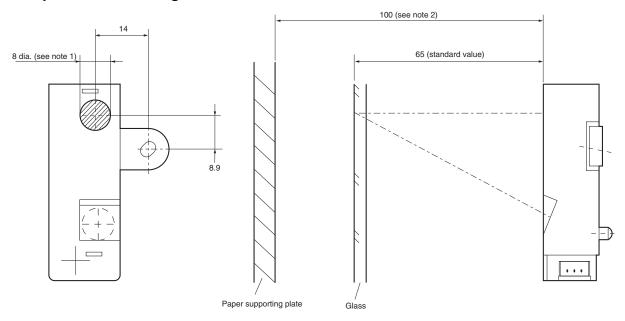
Note: 1. The part with oblique lines indicates the paper sensing area of the EY3A-106-A which is practically determined by the diameter of the beam and its tolerance.
