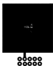
Figure 4. 1 Square Inch of 2-ounce copper
