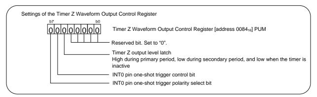
When the timer Z starts counting, the device outputs a high during the primary period and a low during the secondary period from P13 (TZOUT), and when the timer Z stops counting, the device outputs a low. The timer Z set values are shown below.
