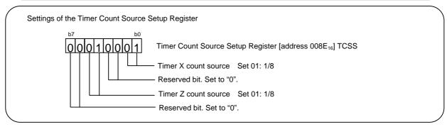
When the respective registers are set up as shown above, the timer X interrupt request bit is cyclically set at 10 ms intervals.
