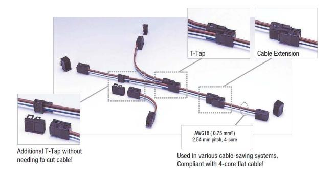
The 3M Link Connector can be used with wire gauges from 18 AWG to 22 AWG and allows different components to be interconnected that may have different wire gauges. The covers are color-coded for proper wire usage. The covers are also designed to increase wire alignment and retention allowing for proper wire termination. Latches and polarization ensure proper mating of the connectors.
