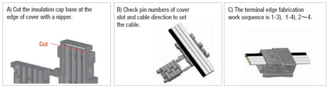
The 3M Link Connector design and termination process allows for easy installation that is capable of cable extension or branching.
