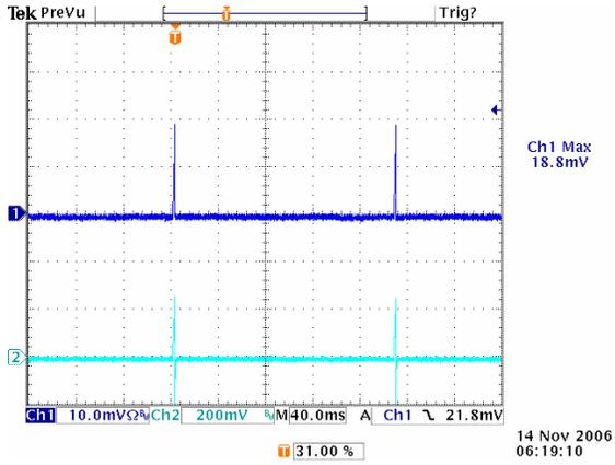
**Figure 25:** Short Circuit Protection at 12Vin, 0.9V out (1mS/div), Ch1: Vo, Ch2: Io, 50A/div
