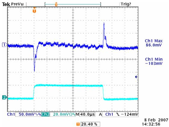
**Figure 21:** Transient Response at 12Vin, 1.8V/40A out (1mS/div)
