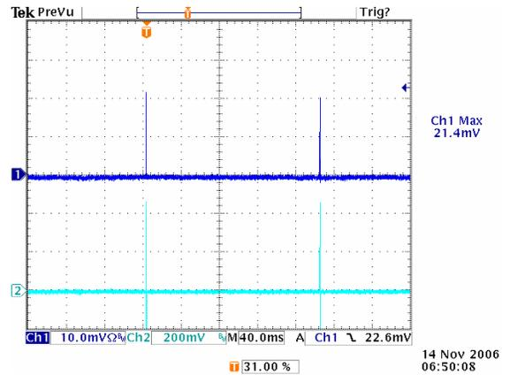
**Figure 30:** Short Circuit Protection at 12Vin, 5.0V out (1mS/div), Ch1: Vo, Ch2: Io, 50A/div
