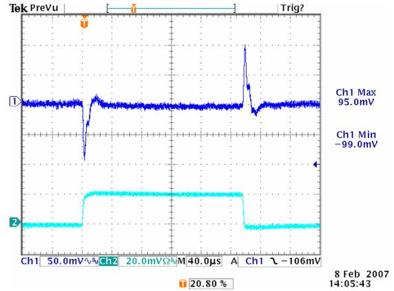
**Figure 20:** Transient Response at 12Vin, 1.2V/40A out (1mS/div)
