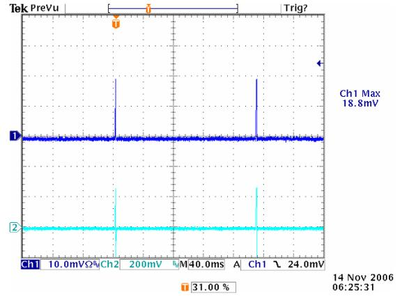
**Figure 26:** Short Circuit Protection at 12Vin, 1.2V out (1mS/div), Ch1: Vo, Ch2: Io, 50A/div
