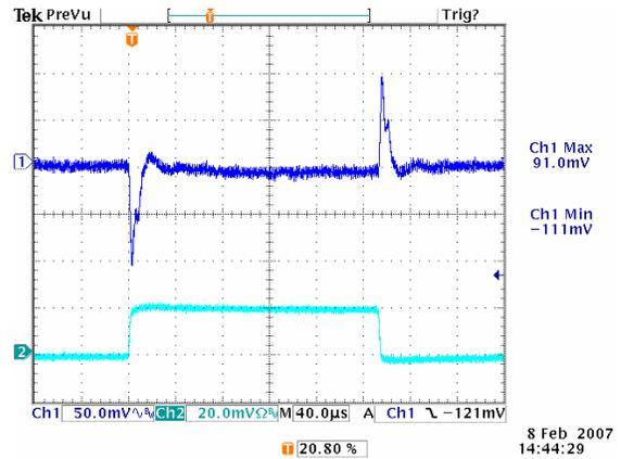
**Figure 22:** Transient Response at 12Vin, 2.5V/40A out (1mS/div)
