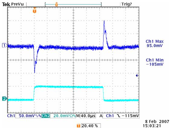
**Figure 23:** Transient Response at 12Vin, 3.3V/40A out (1mS/div)
