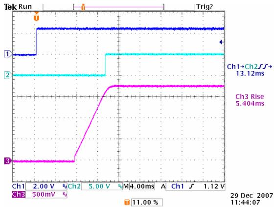
**Figure 15:** Turn on delay time at 12Vin, 1.8V/40A out (1mS/div)
