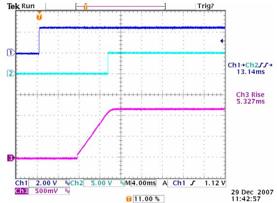
**Figure 14:** Turn on delay time at 12Vin, 1.2V/40A out (1mS/div)
