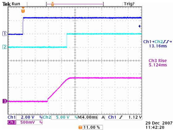
**Figure 13:** Turn on delay time at 12Vin, 0.9V/40A out (1mS/div)
