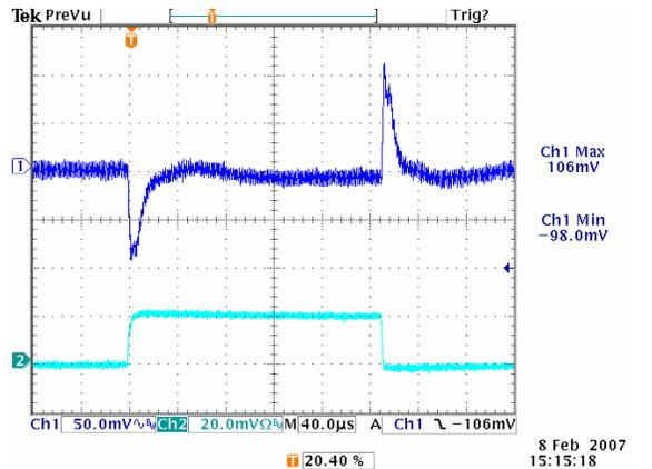
**Figure 24:** Transient Response at 12Vin, 5.0V/40A out (1mS/div)
