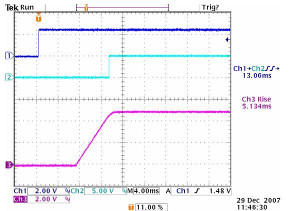
**Figure 18:** Turn on delay time at 12Vin, 5.0V/40A out (1mS/div)
