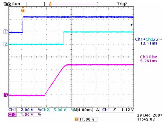
**Figure 16:** Turn on delay time at 12Vin, 2.5V/40A out (1mS/div)
