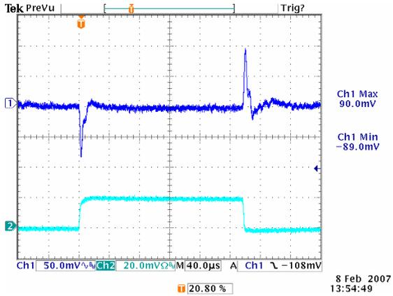
**Figure 19:** Transient Response at 12Vin, 0.9V/40A out (1mS/div)
