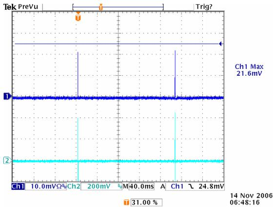
**Figure 29:** Short Circuit Protection at 12Vin, 3.3V out (1mS/div), Ch1: Vo, Ch2: Io, 50A/div
