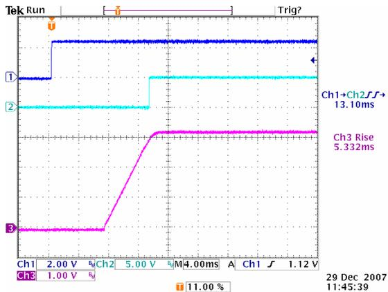
**Figure 17:** Turn on delay time at 12Vin, 3.3V/40A out (1mS/div)
