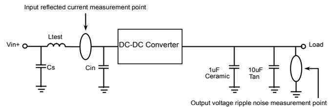
$C_s=330\mu\text{F OS-con cap x1}$ ,  $L_{test}=1\mu\text{H}$ ,  $C_{in}=330\mu\text{F OS-con cap x1}$
