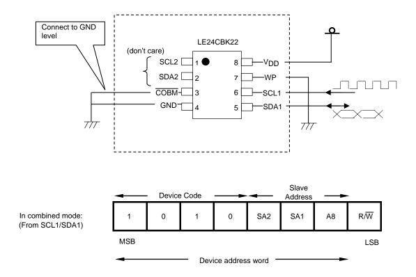
In combined mode, the slave address (SA2, SA1) is don't care, and any combination can be entered (SA2 = 1, SA1 = 1 or SA2 = 1, SA1 = 0 or SA2 = 0, SA1 = 1 or SA2 = 0, SA1 = 0).
