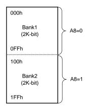
The MSB address in combined mode is A8. A8 is used to select the Bank1 or Bank2 area. Set A8 = 0 to control the Bank1 area, or A8 = 1 to control the Bank2 area.
