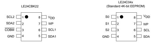
Pin 3 of standard 4K-bit EEPROM products is assigned a slave pin (S2), but Pin 3 of the LE24CBK22 is assigned the COBM pin. Combined mode is entered by setting the COBM pin low. In combined mode, the state of the SCL2 pin and SDA2 pin is "don't care" (may be either high, low, or open).
