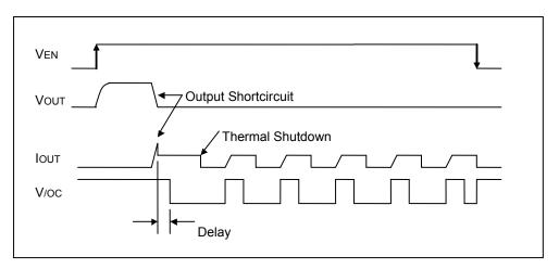
Fig.42 Over-current detection, Thermal shutdown timing (BD2246G)
