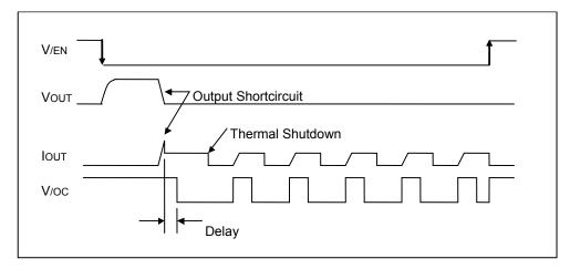
Fig.43 Over-current detection, Thermal shutdown timing (BD2247G)
