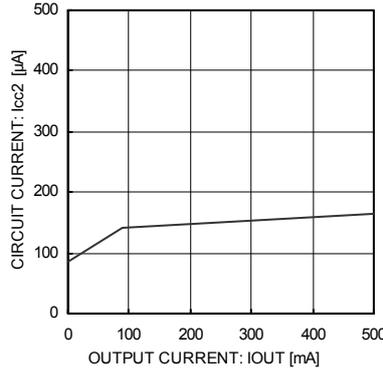
Fig.2 Circuit Current
