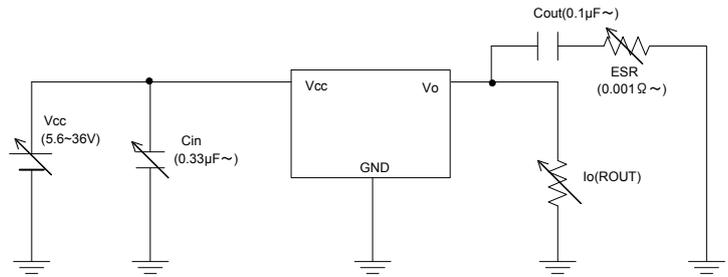
※Pin Settings / Precautions 2 Measurement circuit
