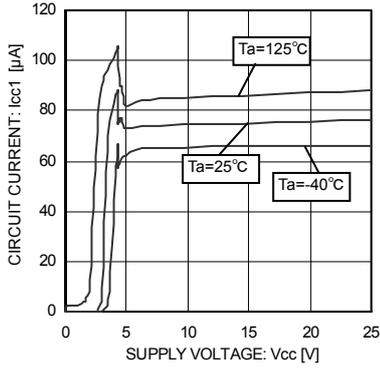
Fig.1 Circuit Current
