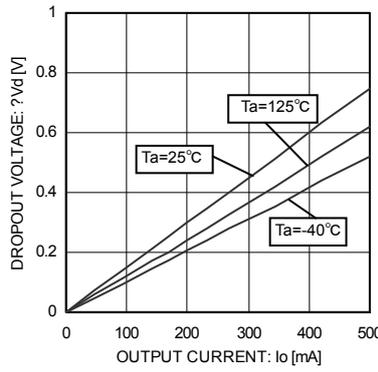
Fig.5 Dropout Voltage
