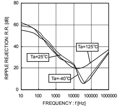
Fig. 6 Ripple Rejection
