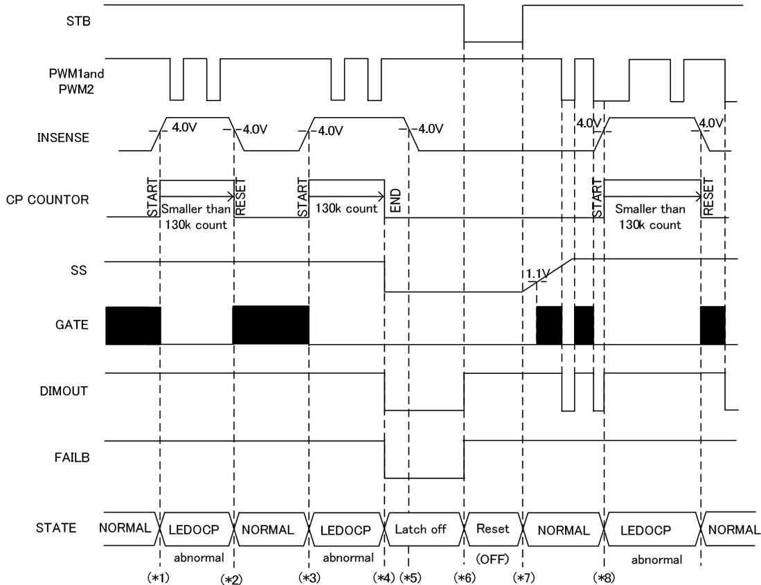
(\*1)...If  $I_{SENSE} > 4.0V$ , LEDOCP is detected, it becomes  $GATE=L$ . To detect LEDOCP continuously, The DIMOUT is compulsorily high, regardless of the PWM dimming signal.
