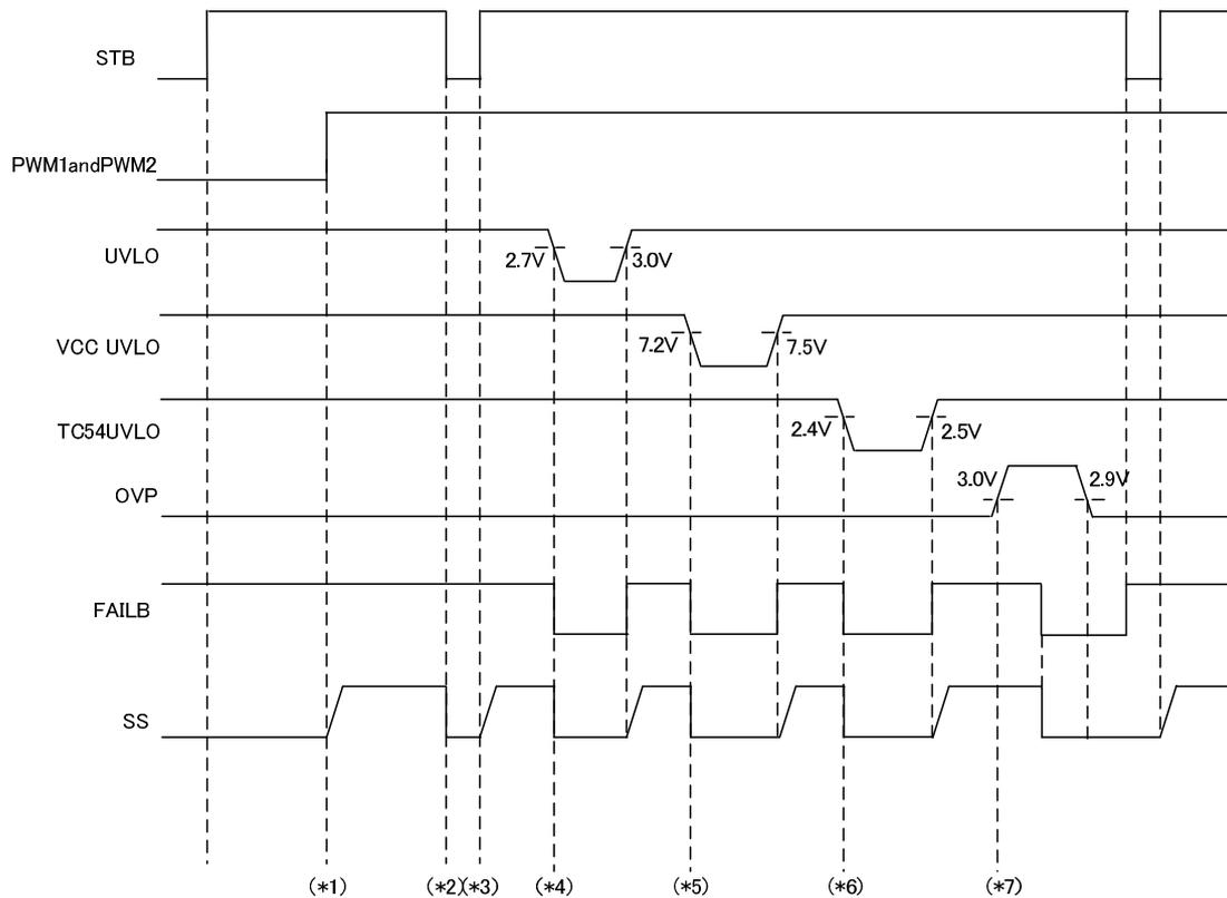
(\*1)...The SS pin charge does not start by just STB=H. "PWM1=H and PWM2=H" is required to start the soft start. In the low SS voltage, the GATE pin duty is depend on the SS voltage. And as the SS is less than 1.1V, the pulse does not output.
