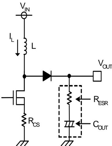
Figure 30. the circuit of the output capacitor
