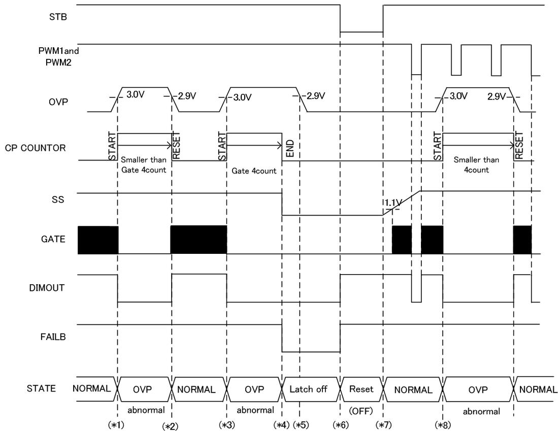
(\*1)...As OVP is detected, the output GATE=L, DIMOUT=L, and the CP counter starts
